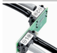
SABIK-NEMBUS-SF Module for operation at constant flow.
